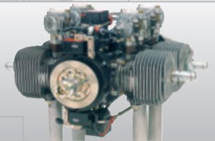
L550 E 2-cycle engine with 37 kW
