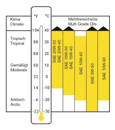
As the temperature ranges of adjacent SAE classes are overlapping, there is no need to change the oil for short time temperature variations. See also information in the section 8.18
