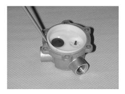
Remove o-ring and strainer from top of pump.
