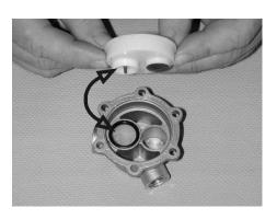
Rotate crankshaft until the diaphragm of the fuel pump is in the lowest position. The plate of the diaphragm (1) is flush with the fuel pump housing (2).
