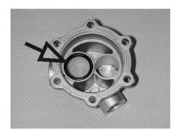
Clean housing. Insert strainer and new o-ring. Insert valve assy until flush with the flange of the cover.
